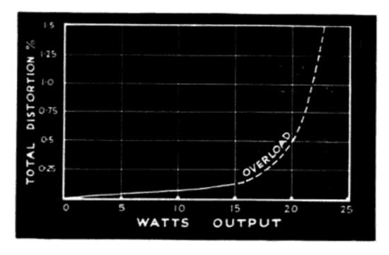
Linearity and overload of the QUAD II power amplifier
